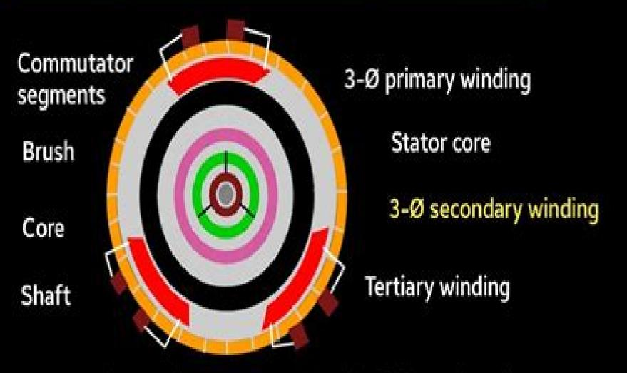
How does Schrage motor works full explanation
