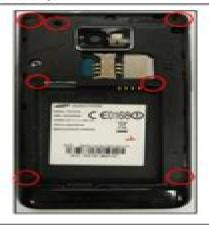
Carefully release the screws at 7 different locations from the rear cover.
