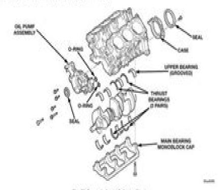
Fig. 70 CremteRaft and Cylinder Block
