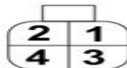
CRANK ANGLE SENSOR CONNECTOR ON DISTRIBUTOR
