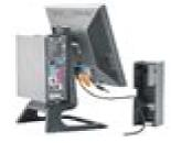
5 Connect the power cable to the manitor as shown.
