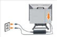
Connect the power cables to an outlet, logish the sable cover.
