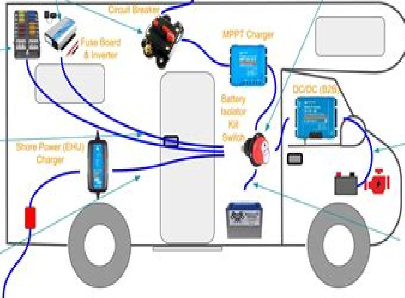
This kill switch is useful to be able to isolate your battery when you park up your rig. This is especially important if you use LiFePO4 batteries to avoid them being charged below freezing temperatures.
