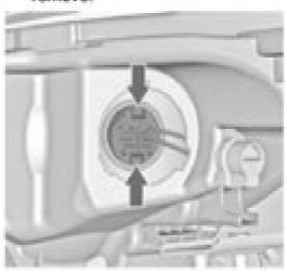
Press latches and withdraw bulb holder from reflector housing.
