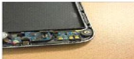
Remove the antenna cable from the main Antenna PCB on the sub-touch key module.
