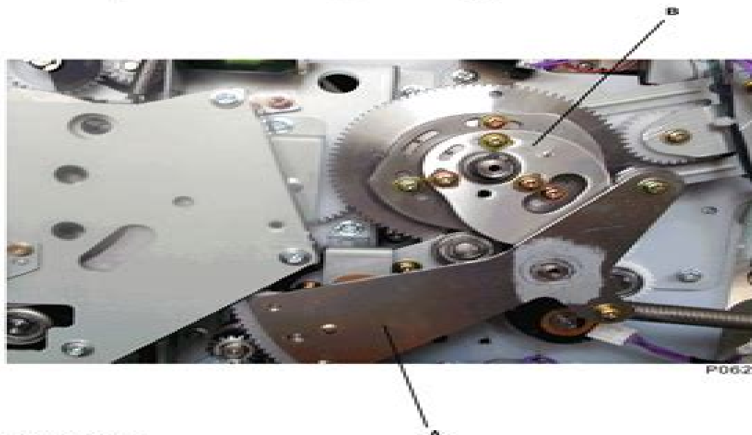
A: Sector-gear assembly B: Timing cam
