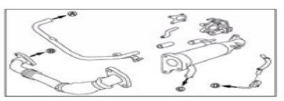
A, C, D: Engine Coolant B: Exhaust Gases
