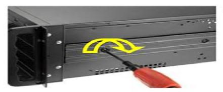
Unscrew all three screws on each side.
