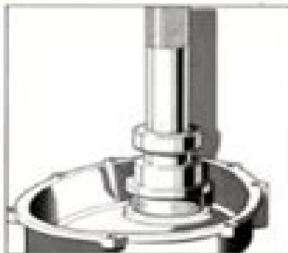
Figure 9 Replacing front cover oil seal
