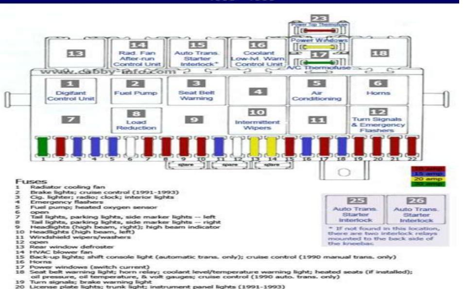
A/C thermofuse: relay position 17 Power window fuse: relay position 17 Power top fuse: relay position 23
