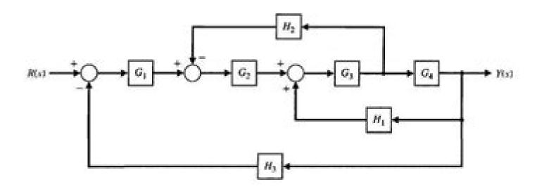
First, to eliminate the loop  $G_3G_4H_1$ , we move  $H_2$  behind block  $G_4$
