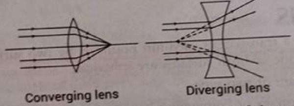
The converging and diverging action of lens can be explained by considering a lens made up of large number of different small angle prisms. In a convex lens, the base of prism is towards principal axis and in concave lens, base of prism is away from the principal axis.
