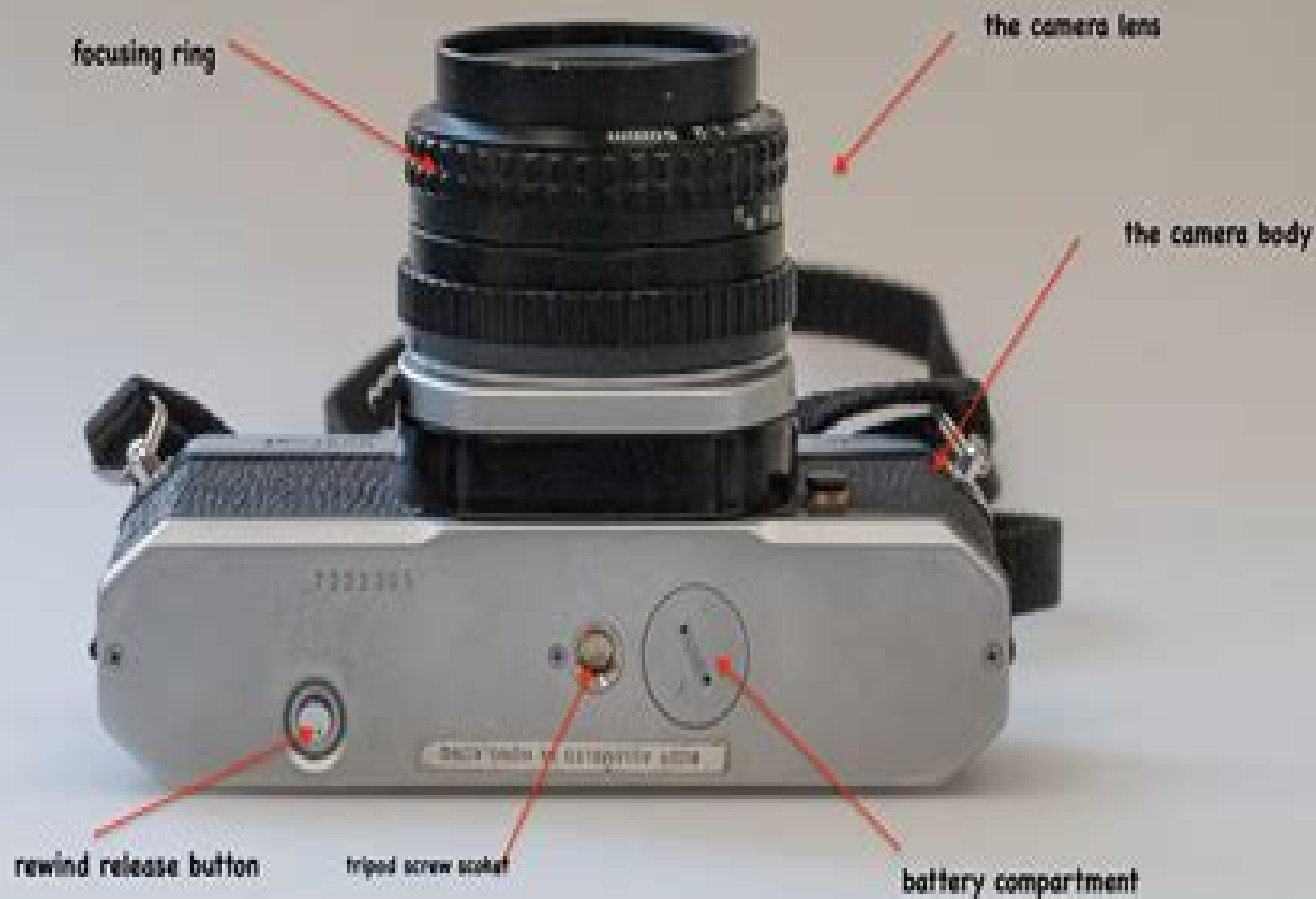
bottom view 35mm mechanical camera
