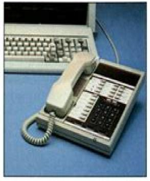
tached to the CBX system to communicate with the outside world. The system includes 512K bytes of memory, two 514-inch disk drives, a 9-inch monitor, and MS-DOS 2.11.
