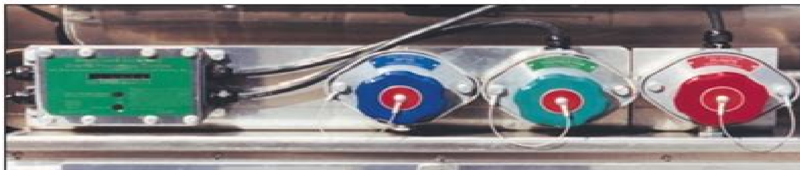
Scully truck mounted control monitor and sockets
