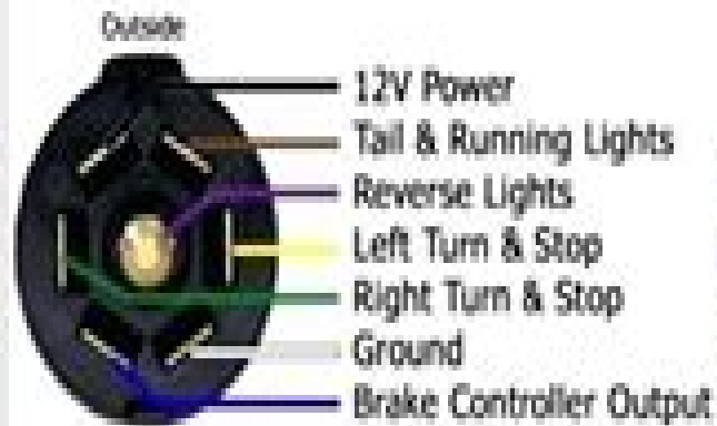
7-Way Traditional (Utility/Equipment/Cargo Trailers)
