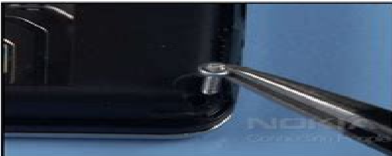
5. Remove the screws.
