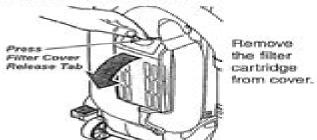
Place new filter cartridge into cover making sure that airflow arrow on side of cartridge points into cover. The foam seal of the filter should be placed against the vacuum cleaner body.
