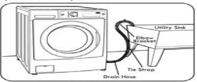
The elbow bracket should be installed near the end of the drain hase. Hang the end of the drain hase over the side of the utility sink. Use a tie strap to secure the drain hase in place.
