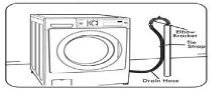
Install the end of the drain hose into the elbow bracket. Do not extend the drain hose more than 4 inches past the end of the elbow bracket. Use a tie strap to secure the drain hose in place.
