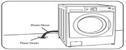
Insert the end of the drain hose into the floor drain.
