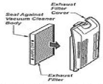
Replace the exhaust filter cover by placing bottom tabs in slots and rotating in until cover snaps into place.
