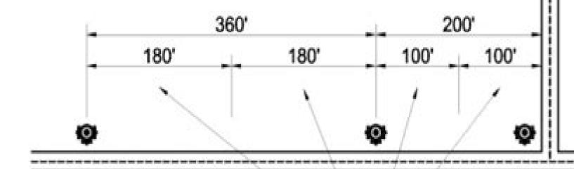
DISTANCE TO HYDRANT LESS THAN OR EQUAL TO 180 FEET - OK
