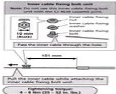
7. Bring the cable around to the cauette joint pulling, hold so that the inner cable fixing nut is facing to the outside thoward the fork end), and then slide the flats part of the inner cable flaing washer into the gap in the pullin.
