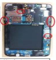
Separate the coaxial cable of antenna assembly from the PBA. Release the screw at 2 points (Size: M1.4\*L3) (Torque: 1.1±0.1 kgf.cm)
