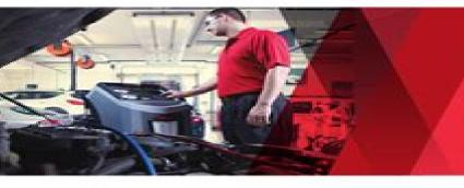
Robinair recovery machines are the North American leaders in R-1234YF service. The AC1234-5 and new AC1234-4 offer fully automatic operation, a powerful 1.5 CFM pump and use a liquid refrigerant flush function to recover more refrigerant faster. Both machines exceed J2843 requirements for R-1234YF recovery, recycle and recharge equipment. Standard features include an integrated refrigerant identifier, automatic internal tank refill, automatic oil drain and a color display.
