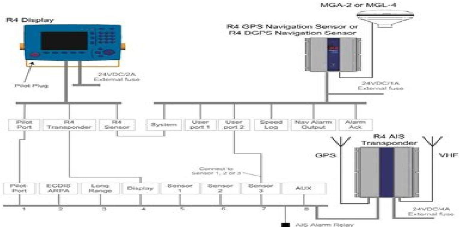
Figure 1-1: R4 Combined AIS & Navigation System overview
