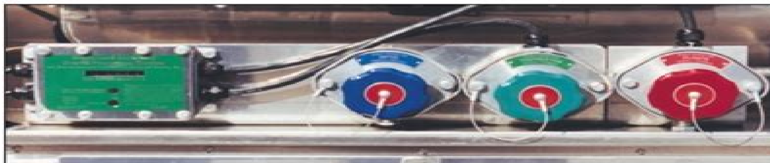
Scully truck mounted control monitor and sockets
