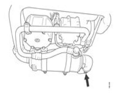
The torque converter must be supported when the power train is raised, see illustration. Replace the rubber cushions on the torque converter with 85x85x40 mm wooden blocks when supporting.
