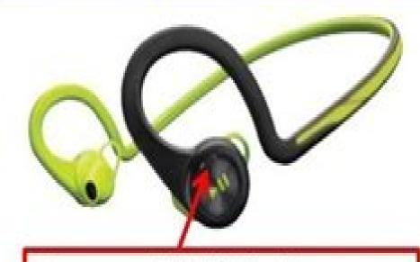
Press and Hold the Power button for 5 or 6 seconds until the LED flashes red and blue.
