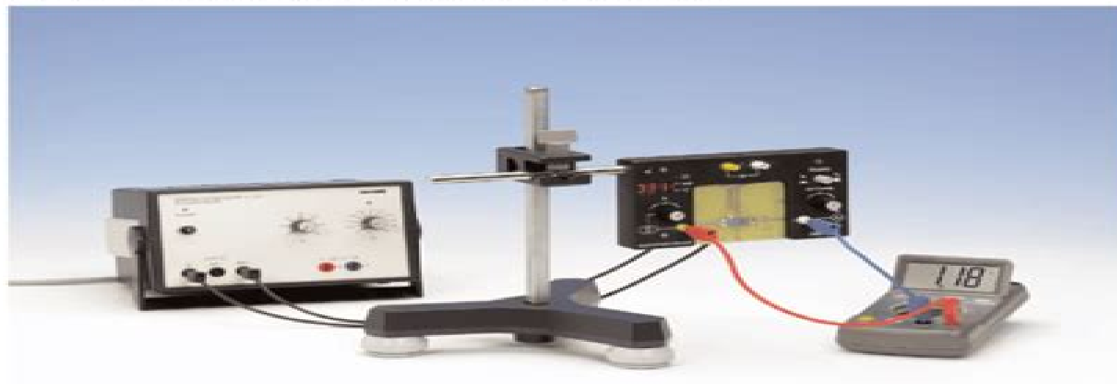
Fig.1: Experimental set-up for the determination of the band gap of germanium
