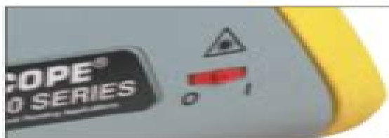
Laser Safety Switch
