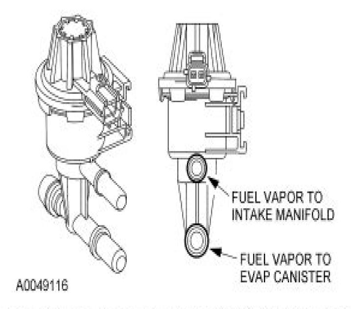
Figure 102: Electronic EVAP Canister Purge Valve
