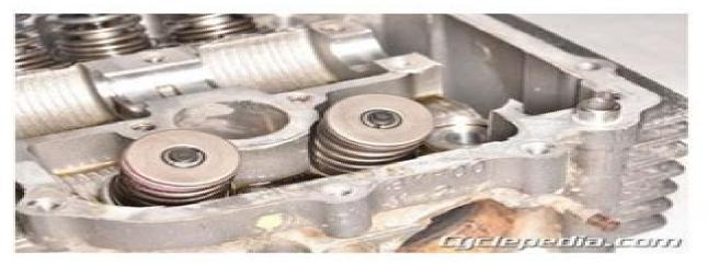
After the valves have been reassemble place a clean shop towel under the cylinder head in the combustion chamber area and gently tap each valve stem with a plastic or rubber mallet to make sure the valves are seated properly.
