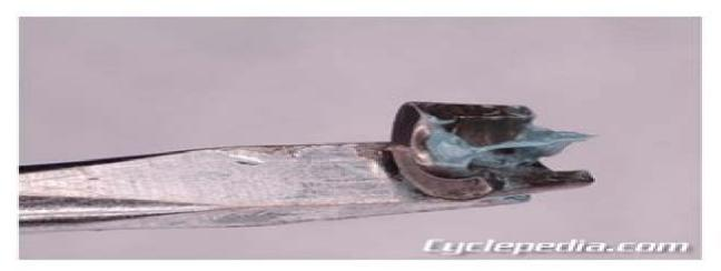
Apply grease to the inside of the split keepers. Apply a dab of grease to the end of a flat blade screwdriver. Set the keeper in the grease on the screwdriver and insert it onto the valve stem. Repeat this with the other keeper.
