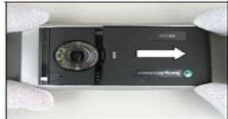
Start to remove the battery from the phone with your fingers. Lift up the battery in the top end to unleash it.
