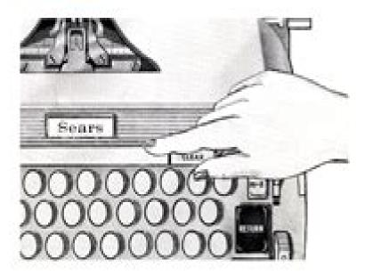
Any time you need to skip the same number of spaces several times in typing, you save time and energy by using the Tab Bar (30). To type columns or indent paragraphs, for example, move the carriage to the desired spot, and depress the Tab SET Key (29). Do this for as many tab stops as you need. Each time you want to type at one of these spots, depress the Tab Bar. The carriage will move to each succeeding stop each time the bar is depressed.
