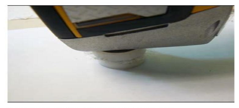
2. Place the analyzer so the sample is covered by the analysis window.
