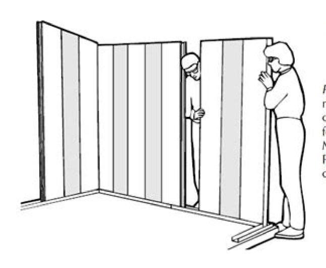
Insert a group of 3 side wall panels labeled JT1-PT1-JT1 into side channel at the right front corner allowing room for a Groove Panel PT1. Make sure a Joiner Panel faces the front corner.
