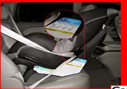
Using the FORWARD-facing belt path for a rear-facing installation:
