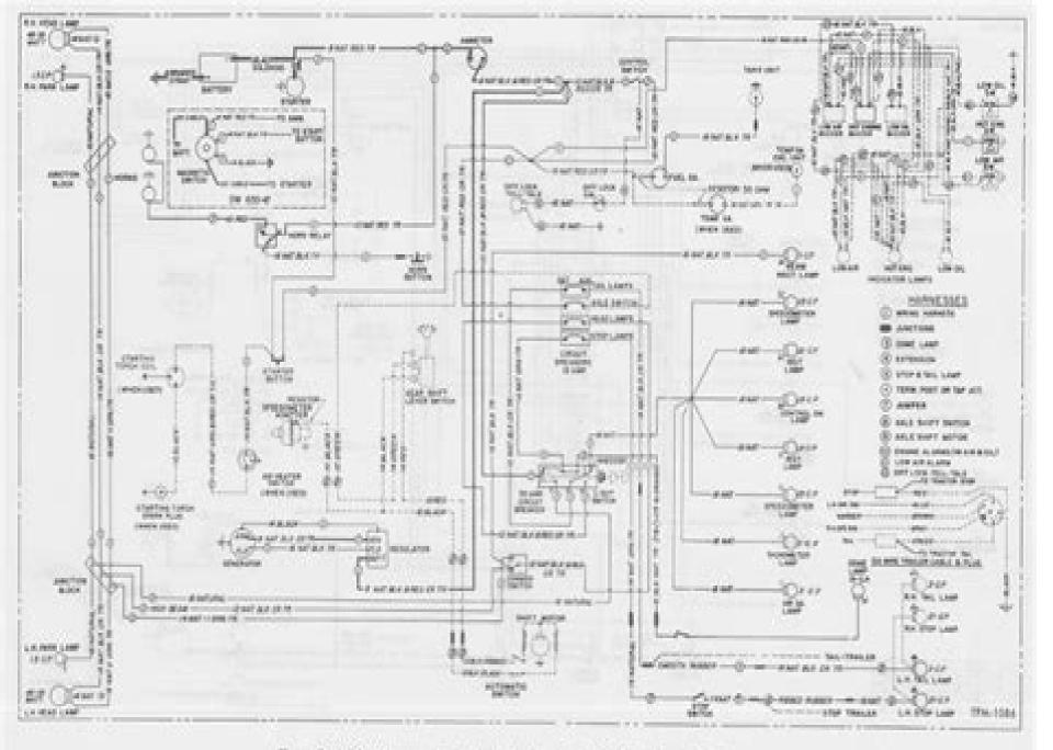
Figure 3—Wiring Diogram—Early Diesel Models—Series D620-47 Through D660-47
