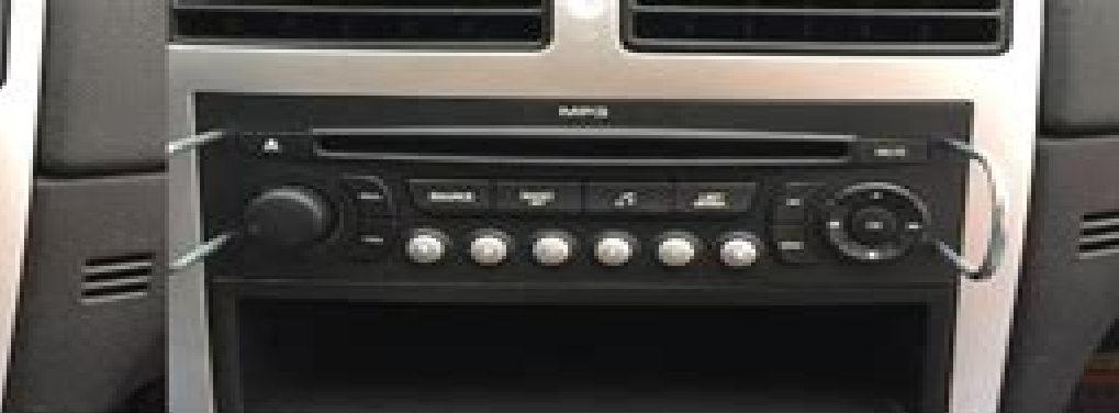
2. USING A U-SHAPED TOOL INSERT IT INTO THE MAIN UNIT REMOVAL HOLE
