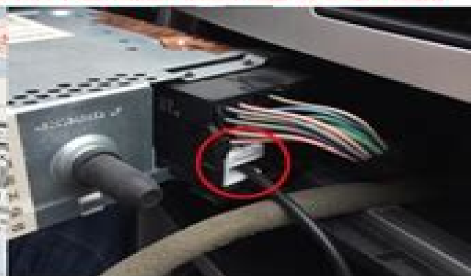
5. INSERT INTO AUX IN PORT
