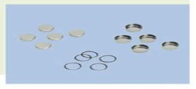
DSC measurement requires that samples are enclosed in a sample pan in order to avoid the direct contact between sample and furnace and/or sensor, because if the samples come into contact with the furnace/sensor problems can occur on the baseline. Memory can be affected and damage to the furnace/sensor can occur (in the worst case the furnace/sensor can be destroyed).
