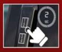
Within five seconds of releasing the "1-2" button, press and hold the "1-2" button for two seconds.
