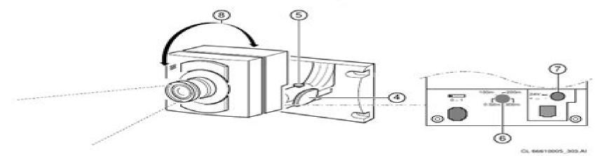
14. Check if the cable length compensation (6) selector is set to the correct length. The length set must be the same as the length of the system cable (0-300m/900ft max.) connecting monitor and camera.
