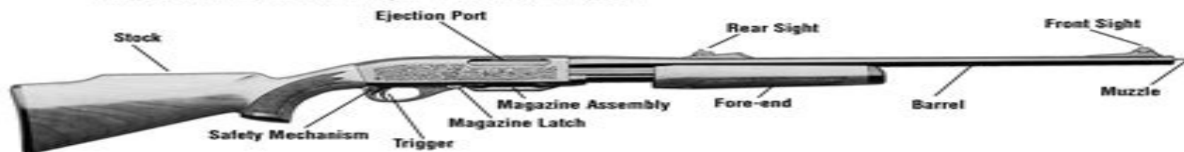
PICTURE 1 This picture shows the main parts of a REMINGTON MODEL 7600™ PUMP ACTION RIFLE. The picture will aid in understanding the instructions in this book.
