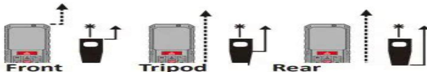
The measuring data should be different due to different Reference settings.
