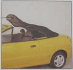
B - Press the front part of switch I until the hood stops moving completely: the hood compartment cover will be locked and the front edge of the hood will stop approximately 14 inches [35 centimetres] from the windscreen.
