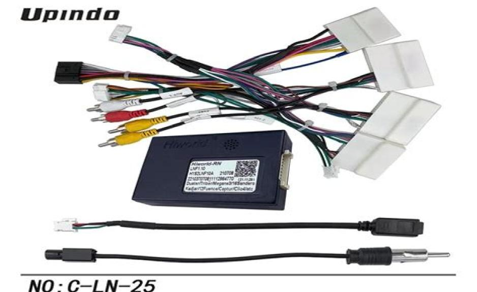
Car Radio Cable with CAN bus Box For Renault Clio4 / Kadjar 2016 / Duster 2019 Arkana 2019
