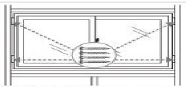
STEP 2. Secure window using 2-1/4" screws fastened through the pre-purched installation holes located on the side walls las shown above.
