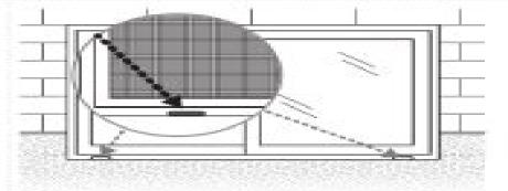
STEP 4. To insure proper water drainage keep weep holes clear and free from obstruction (see above).
