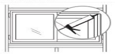
STEP 3. Fill the gags, interior, exterior and around the perimeter of the window between the mainframe and wall with an approved polyurathene based sealant such as Vulkem® or 100% silicone window and door saals.
